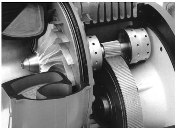
**FIGURE 4.19** Cutaway view of a turbo compressor showing the gear box, the impeller, and the discharge diffuser vanes in open position. (From HV-Turbo A/S, Denmark. With permission.)
